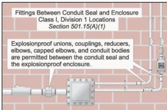
Electrical "Y-Seal", (EYS) prevent explosions from spreading through conduit systems and igniting outside atmospheres. When properly installed and filled with a UL-listed sealing compound, they create a physical barrier that minimizes passage of explosions from traveling freely through the conduit.
